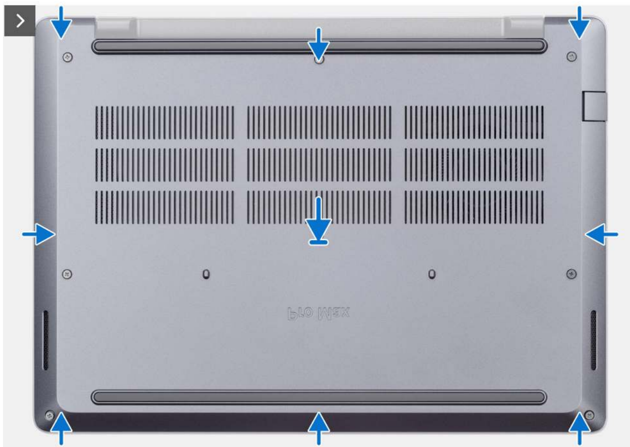
Abbildung 14. Installing the base cover
