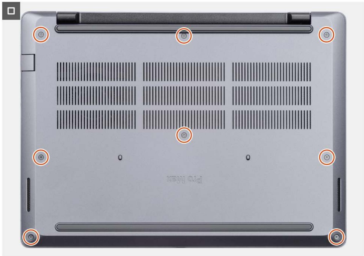
Abbildung 15. Installing the base cover
