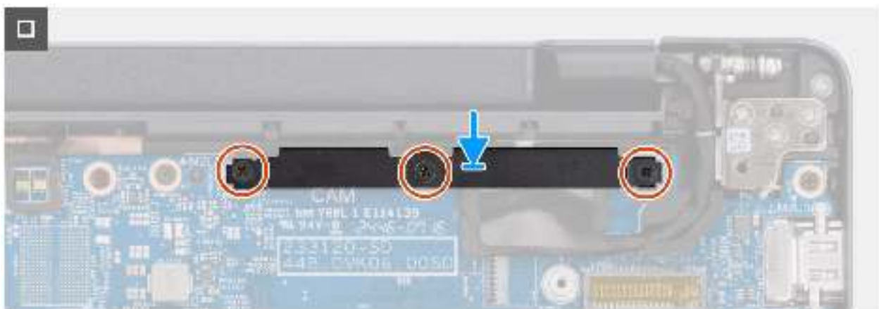
Abbildung 85. Installing the system board
