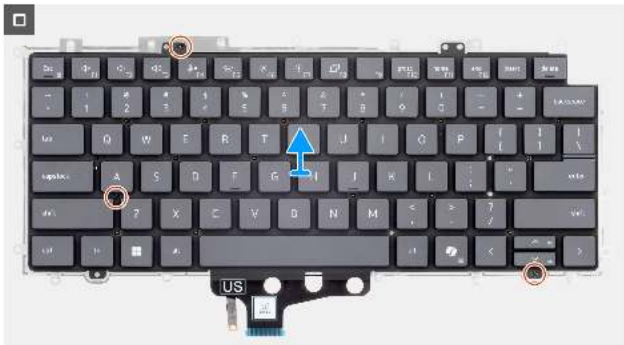
Abbildung 96. Removing the keyboard
