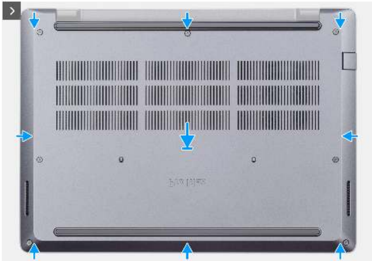
Abbildung 14. Installing the base cover
