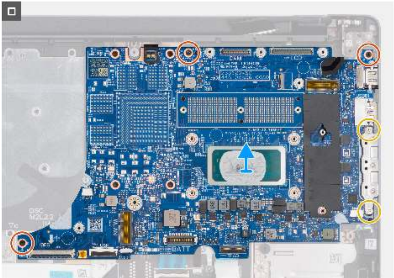
Abbildung 79. Removing the system board
