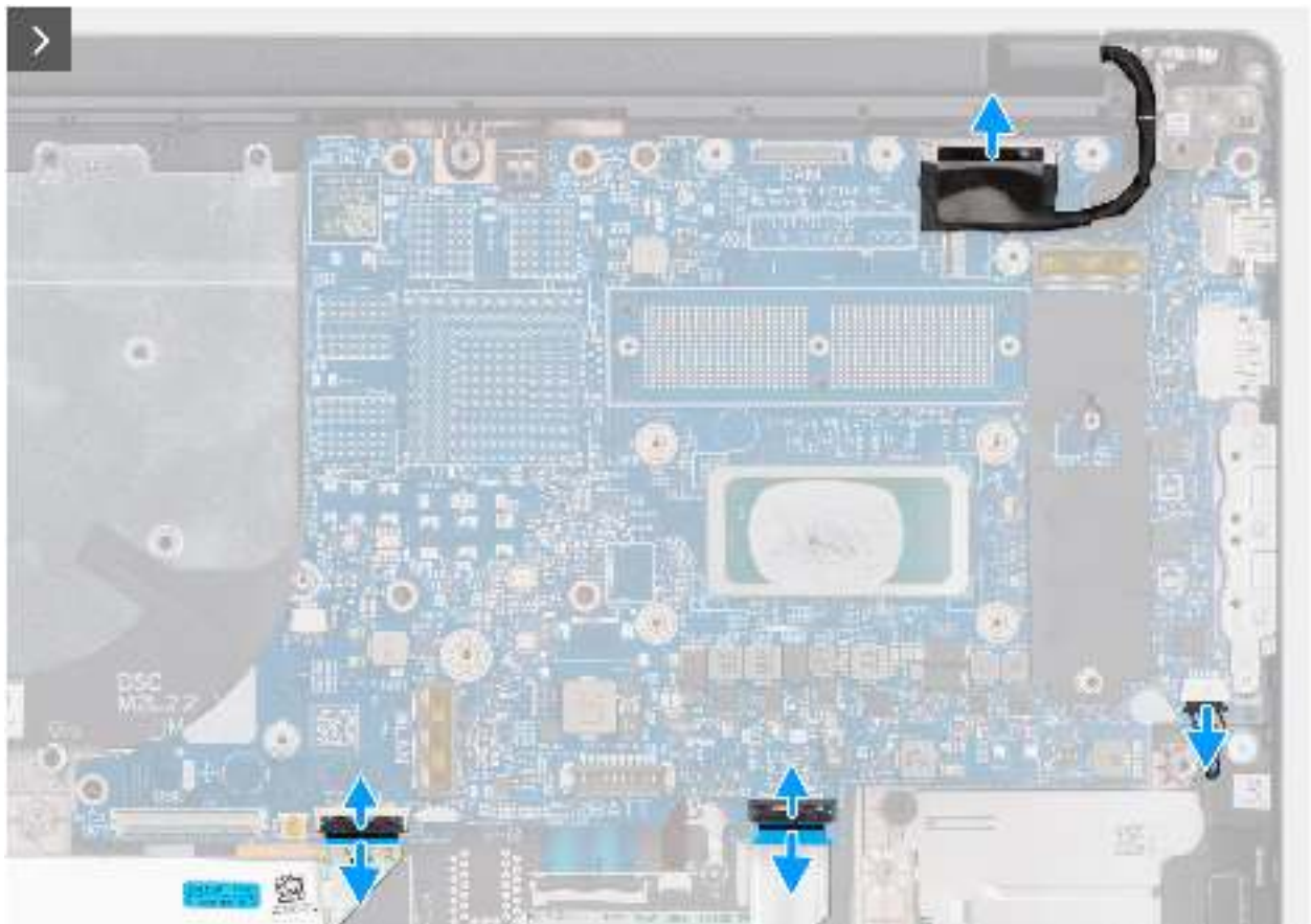
Abbildung 78. Removing the system board
