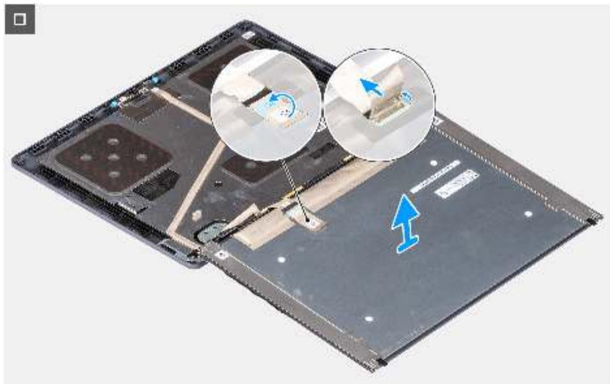
Abbildung 62. Removing the display panel
