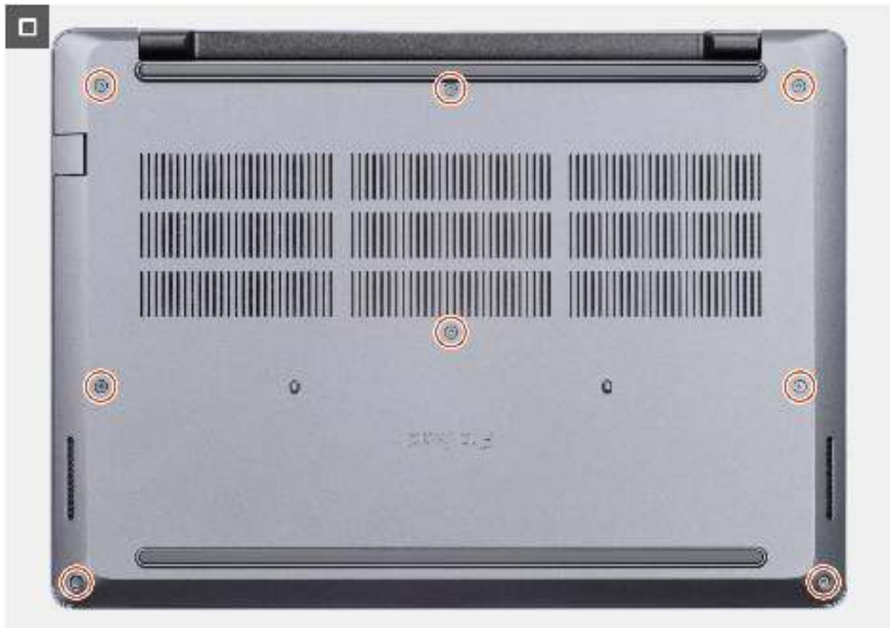
Abbildung 15. Installing the base cover
